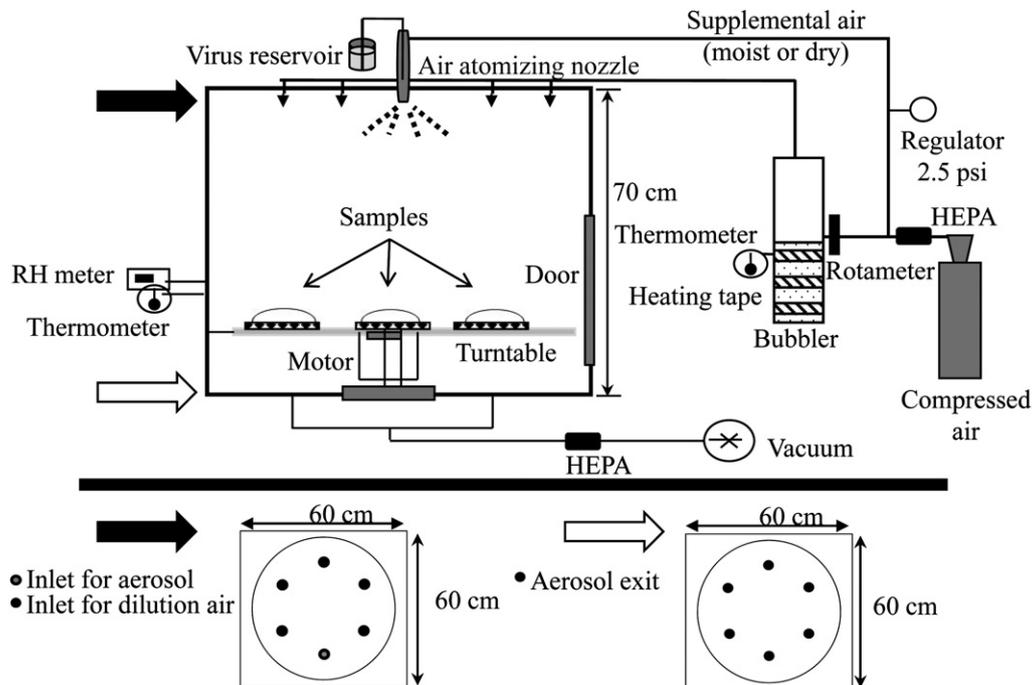
**Fig 3.** The droplet loader device used to apply droplets to the FFRs. The device is composed of a stainless steel shell (60 cm l × 60 cm w × 90 cm h). Droplets are created by applying compressed air to an air-atomizing nozzle that produces a droplet at the source with a CMD of ~40 μm. Uniform dispersion of the droplets onto the test specimens is achieved by rotating the samples on the turntable at 3 rpm.
