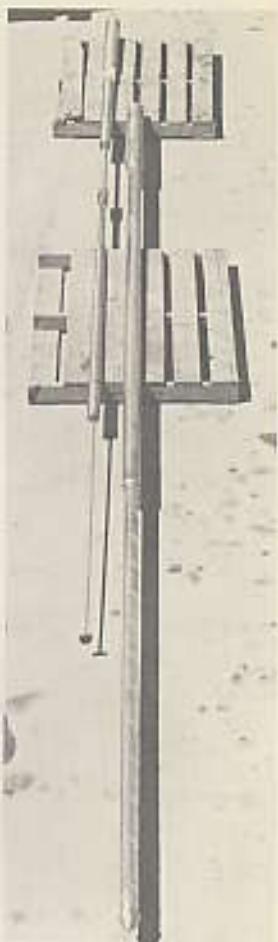
24 Control Element, disassembled. The right-hand rod is the thimble into which the control element is fitted. The neutron absorbing material is made up of 18 rings of boron-nickel alloy. There are a total of four control elements in the reactor, each of which controls 1.6 per cent of reactivity. Drive motors are capable of controlling the movement of the control elements at speeds of either 0.24 or 3.0 feet per minute.
