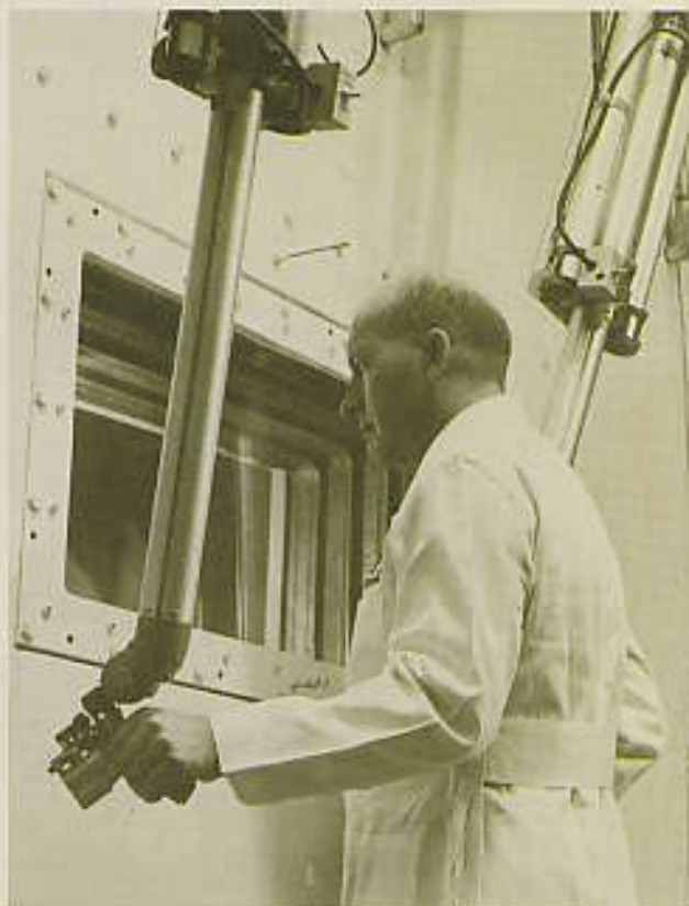
56 Hot Cell Manipulators. The operator observes the experiment through 42 inches of lead-glass plates. The hot cell, located below floor level at one end of the reactor room, is equipped with three sets of manipulators and viewing windows, and provides a facility for the examination of any radioactive components removed from the reactor.
