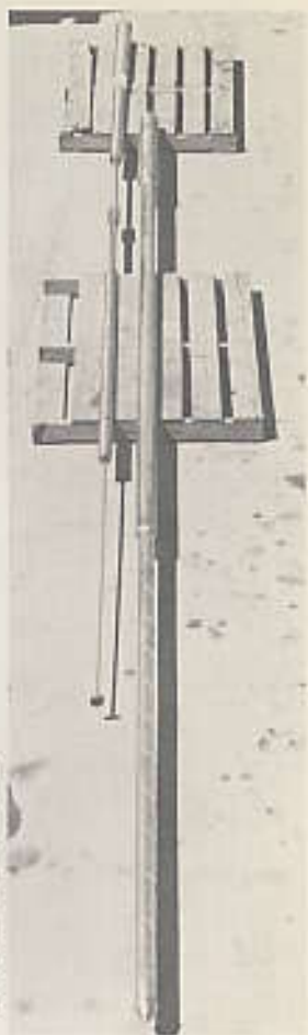
24 Control Element, disassembled. The right-hand rod is the thimble into which the control element is fitted. The neutron absorbing material is made up of 18 rings of boron-nickel alloy. There are a total of four control elements in the reactor, each of which controls 1.8 per cent of reactivity. Drive motors are capable of controlling the movement of the control elements at speeds of either 0.24 or 3.0 feet per minute.
